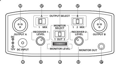
Balanced Audio Output Jack: TA3M-type connector. Pin 1: ground (shield); Pin 2: "audio +"; " Output A Pin 3: "audio -". Use the included TA3M to XLRM interface cable to connect the receiver output to a balanced microphone-level input on a camera, mixer or integrated amplifier.
